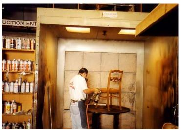
Figure 2-2. Typical Spray Booth at Wood Coating Operation
