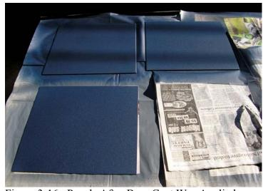
Figure 3-16. Panels After Base Coat Was Applied
