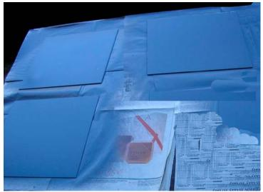
Figure 3-15. Panels After Primer Was Applied
