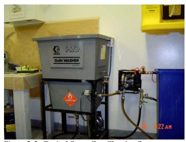
Figure 2-5. Typical Spray Gun Cleaning System
